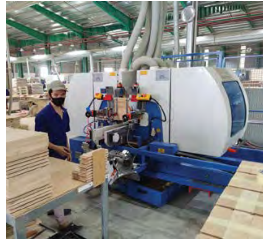
Worker Cutting Dovetails with Precision Jig
